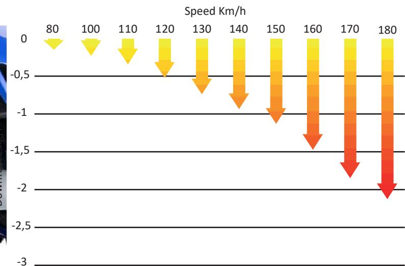
The Downforce that the spoilers generates raises potentially as the speed increases, at 180km/h we get 2.11 Kg/f.
